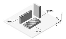
The FDM process creates parts with a layered structure, causing mechanical properties to be anisotropic based on print orientation.\*1
